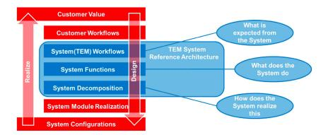
Capella has been chosen to implement this approach. With its native support of a Model-Based Systems Engineering (MBSE) method, and used with a system decomposition approach, Capella makes it easier to maintain consistency in the design of the systems. It also increases automation opportunities by leveraging the model's digital format.
